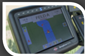
SprayRover 570 GPS controlled AutoSectionControl
